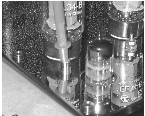
Showing a probe in output valve test point
