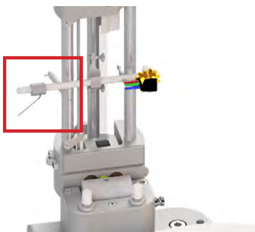
Pic. 21: Fixing the counterweight
