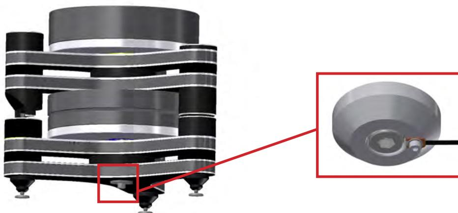
**Pic. 5:** Grounding the bearing
