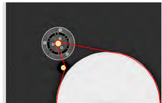
Pic. 3: Mounting the drive belt
