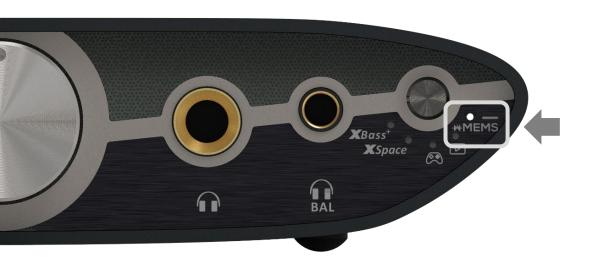
ZEN CAN 3 now supports IEMs using **xMEMS** technology, an innovative speaker technology pushing the boundaries of headphone performance.
